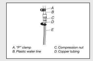
6. Check connection by pulling on copper tubing. Attach copper tubing to refrigerator cabinet with a "P" clamp. Turn on water supply to refrigerator and check for leaks. Correct any leaks.
